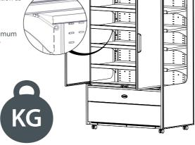
Do not block air vents with product. A minimum of 25mm should be maintained between the top of the product and the shelf above.
