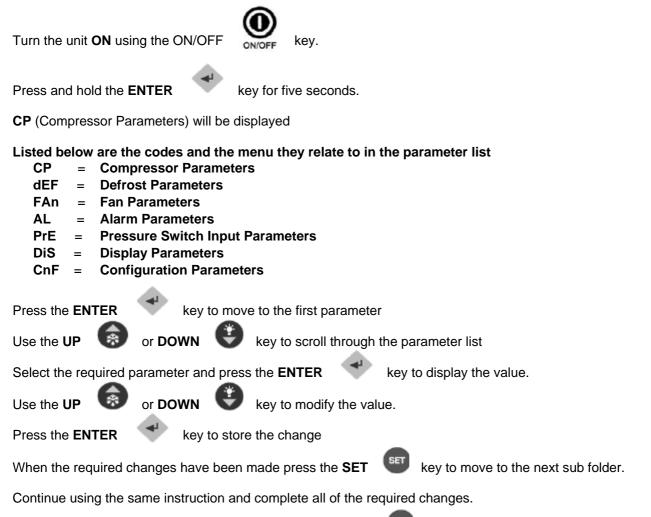
Once all of the changes have been completed press the **SET** key twice or wait for ten seconds to return to the temperature display screen.
