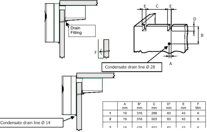
1 SP101HW - 201HW - 301HW - 101LW 2 SP401HW - 501HW - 201LW 3 SP601HW - 301LW \*NOTE: Dimension for 75mm insulation increase by 24mm if 100mm insulation is used. On low temperature models a drain line heater is inserted into the drain fitting.
