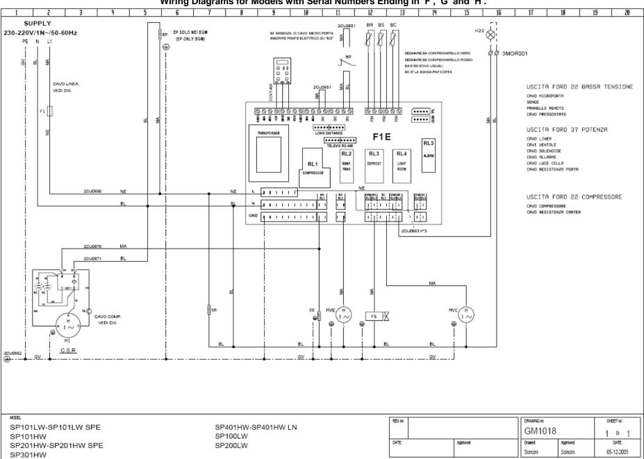
Wiring Diagrams for Models with Serial Numbers Ending in 'F', 'G' and 'H'.
