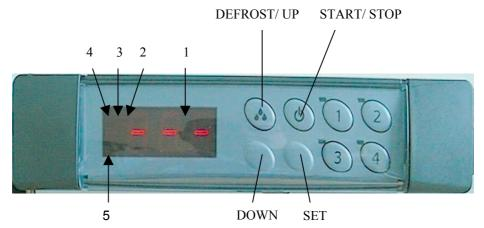
**Display Set Point**: Press the SET key whilst in the HOLD Mode will display the set point for 5 seconds.
