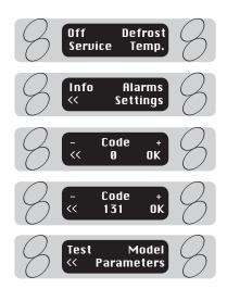
From 'Service Main Menu' press button 4 (<<) to exit to 'User Main Menu'. If no further buttons are depressed for one minute the controller will also revert to the 'Normal Operating Mode'.
