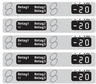
From 'Output Relay Test Menu' pressing button 4 (<<) will cause the controller to return to the 'Service Main Menu'. If no buttons are depressed for one minute the controller will revert to the 'Normal Operating Mode'.
