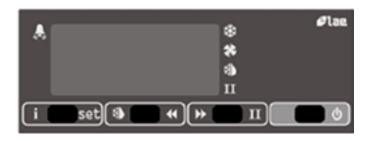
Controller with the LCD 16 Display (00-555740) fitted as from May 2007 to November 2007 Controller display LCD5s (00-555992) fitted as from November 2007
