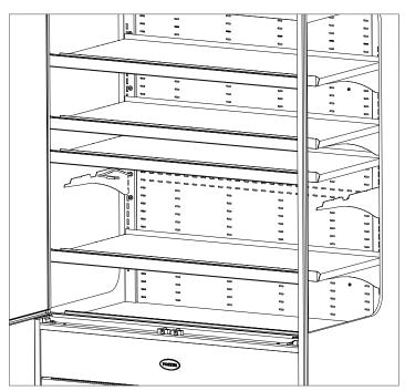
4 Position the shelf support brackets at the desire location. Ensure that the shelf support brackets are engaged correctly. Both locating points should be fully engaged with the vertical rail as shown.
