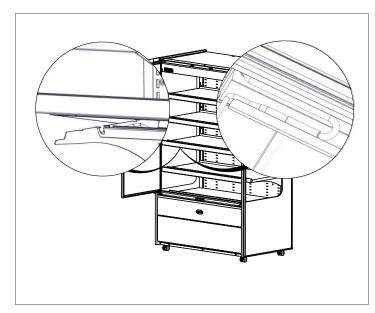
**2** Disconnect the connector for the shelf light. Lift the shelf from the shelf support brackets and support while the brackets are re-positioned.
