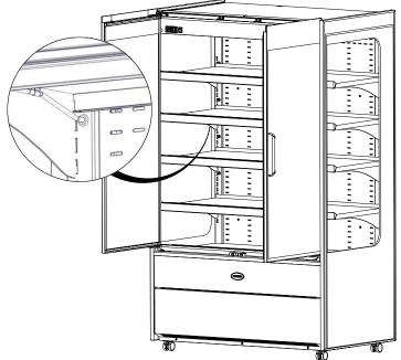
Do not block air vents with product. A minimum of 25mm should be maintained between the top of the product and the shelf above.
