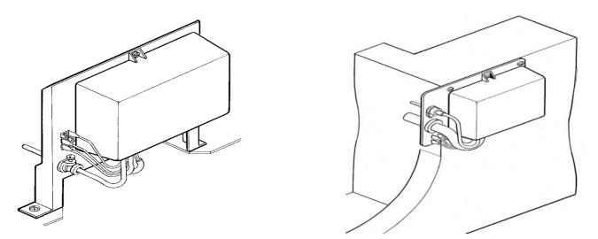
Fig 2A Single Section Top Mount
