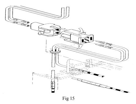
For the correct fitting arrangement see following page for frame heater layout. Replace the heater.
