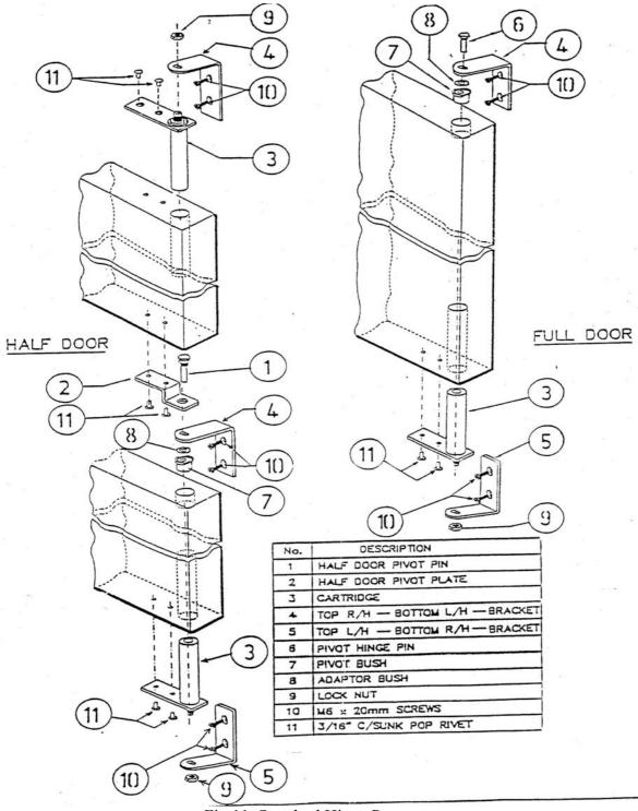
Fig 11. Standard Hinge Parts.
