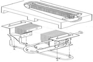
Fig 9A. Single section Evaporator
