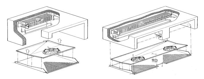
Fig 7A. Single Section Evaporator Housing.
