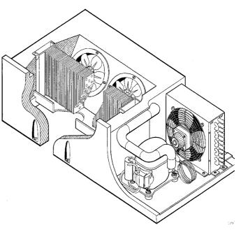
Fig 4A Single Section Plug Box.
