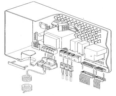
Fig 1. Power Switching Unit.
