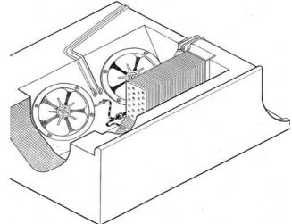
Fig 6A Single Section Top Mount.
