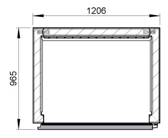
3.4 Ceiling panel with the refrigeration system / heater assembly
