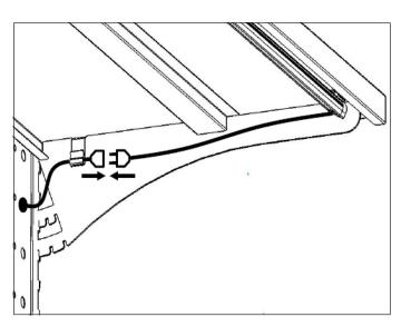
Plug the LED into the clipped cable tree branches.
